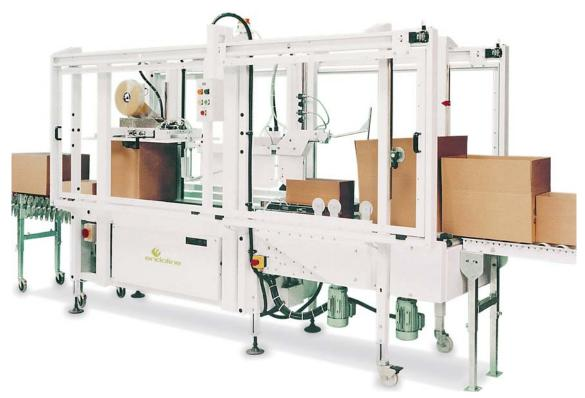
This is the dominant machine of its type having originally been developed for the biscuits and snack foods industries. It automatically adjusts to random sizes while sealing small and large, lightweight and heavy cases without the need for an operator. It is fully automatic and provides secure and accurate taping at speeds of up to 14 cases per minute. Fully automatic random sealing machines are ideally suited to applications where there is insufficient room for a sealer on each packing line.
